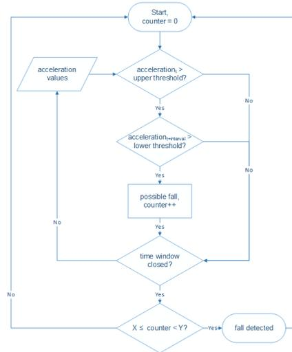
Fig. 2. Fall detection algorithm.
