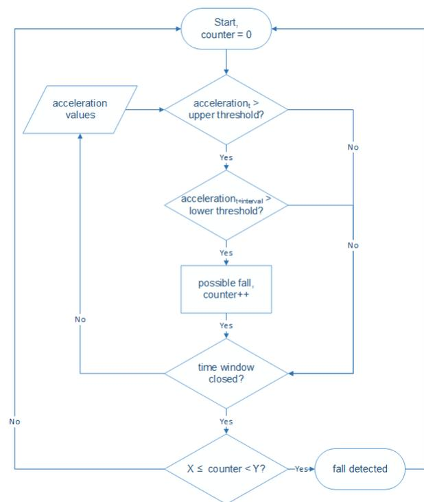
Fig. 5. Fall detection algorithm.
