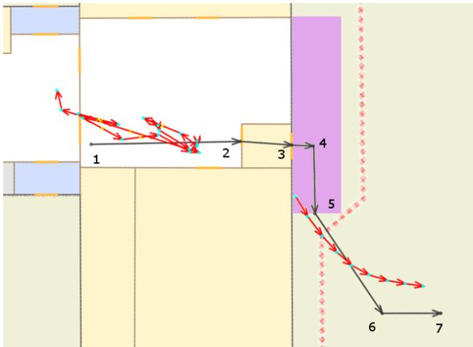
Fig. 5. Estimated positions using the switching algorithm, are shown in red (indoors and outdoors). The true trajectory of the user appears in grey.
