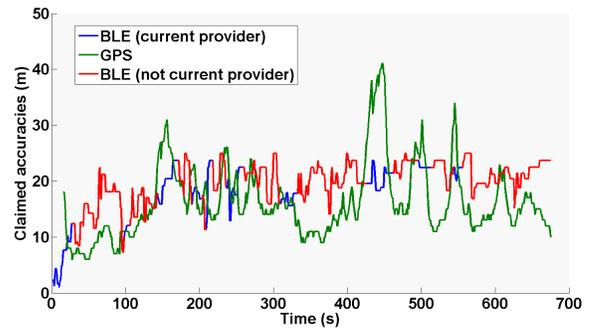
Fig. 6. Claimed accuracies of GPS (green line) and BLE (blue when BLE is the current provider, red otherwise), received at the limit of indoor/outdoor areas.
