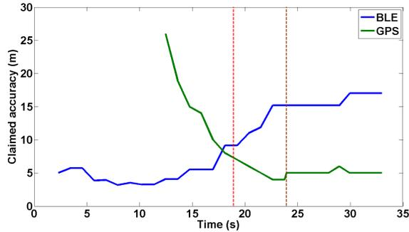
Fig. 4. Claimed accuracies of Bluetooth (blue line) and GPS (green line), during a movement from indoor to outdoor environment. The dashed lines indicate the moment that the user went outdoors (red dashed line), and the moment the provider switched (brown dashed line).
