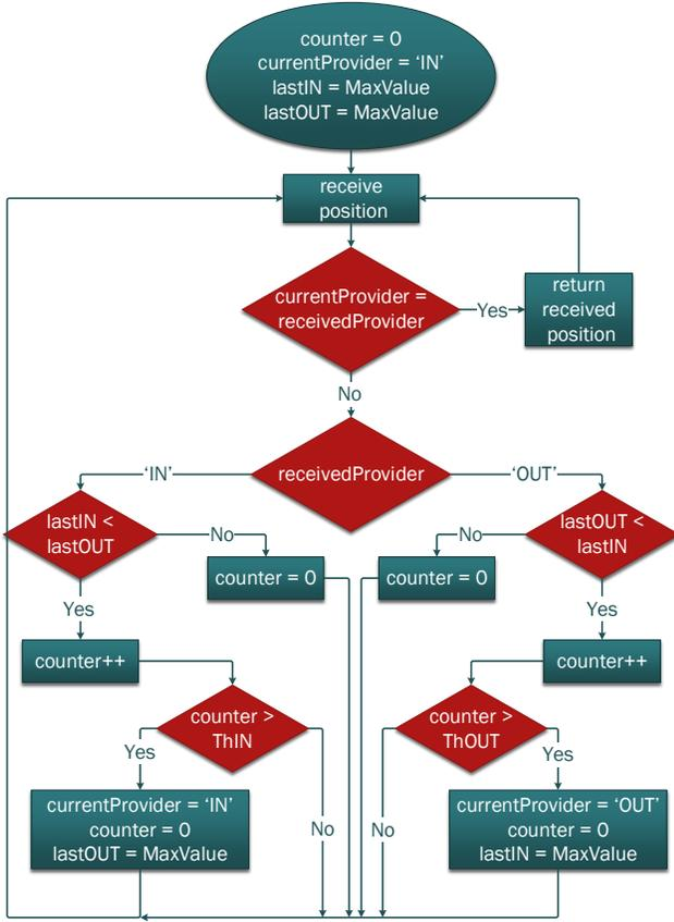
Fig. 3. Flow chart of switching algorithm
