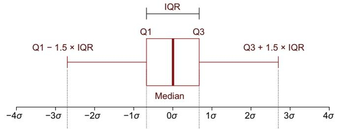
Fig. 2. Example of a box plot.
