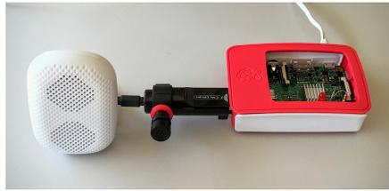
**Figure 6:** The implemented prototype comprises a commodity speaker and a microphone connected to a Raspberry Pi board.
