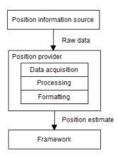
Figure 2. Transformation of raw output data to formatted position estimates.
