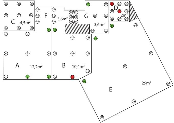
Fig. 5. House evaluation area and targeted locations (green for the points with an error improvement, red for an error deterioration).
