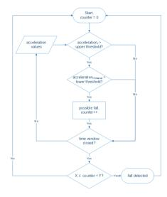
Fig. 2. Fall detection algorithm.
