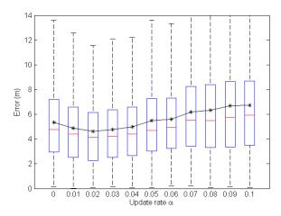
Fig. 3. Box plot and mean values (black line) of the positioning error for several values of the update rate  $\alpha$ , using a Samsung Galaxy S5.
