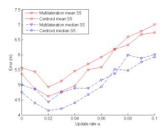
Fig. 4. Mean and median values of the positioning error using multilateration and weighted centroid, for several values of the update rate  $\alpha$ , using a Samsung Galaxy S5.
