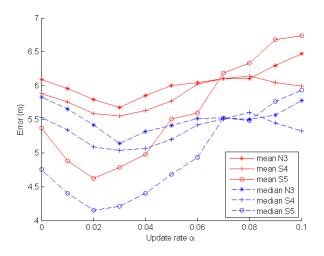
Fig. 2. Mean and median values of the positioning error of the three devices used, for several values of the update rate  $\alpha$ .
