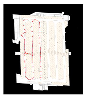
Fig. 1. The path followed in the parking. The area where coverage is provided is the left half side of the parking, and its dimensions are 120 by 40 m.
