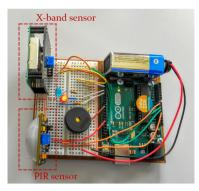
Figure 8: Circuit used to test the PIR and the X-band sensors.
