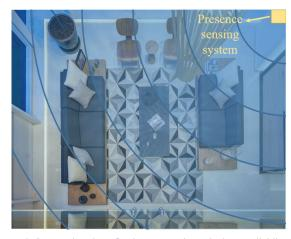
Figure 5. Segmenting the reflection pattern is equivalent to dividing the environment into segmented spaces (iteratively discarding the first i segments).
