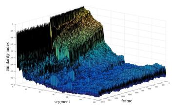
Figure 8. Similarity indices over segmented reflection patterns for vacant (frames 1-1000) and occupied environment (frames 1001-2000), case of high SNR, Room A, LOS.
