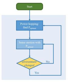
Fig. 3 Flow chart showing how the power hopping is triggered when the environment is changed
