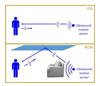
Fig. 1 A different transmitter power is required in each case
