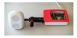
Fig. 7 Prototype of the ultrasound motion sensor used for testing
