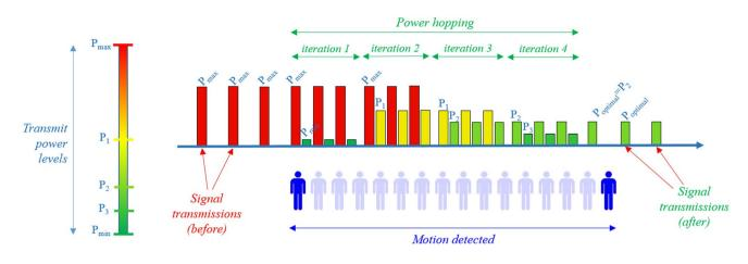
Fig. 2 Power hopping example: adapting to the optimal transmitter power level
