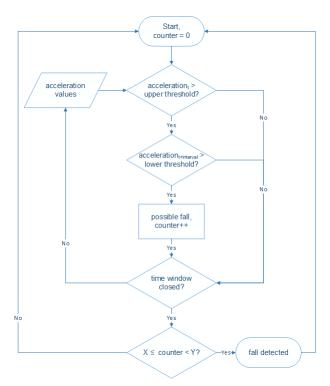
Fig. 5. Fall detection algorithm.
