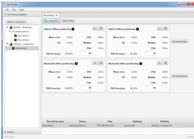
Fig. 5. The interface of the GpmStudio tool suite.
