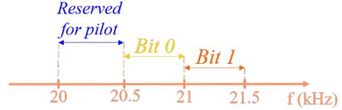
Fig. 4. Frequency allocation of chirp signals
