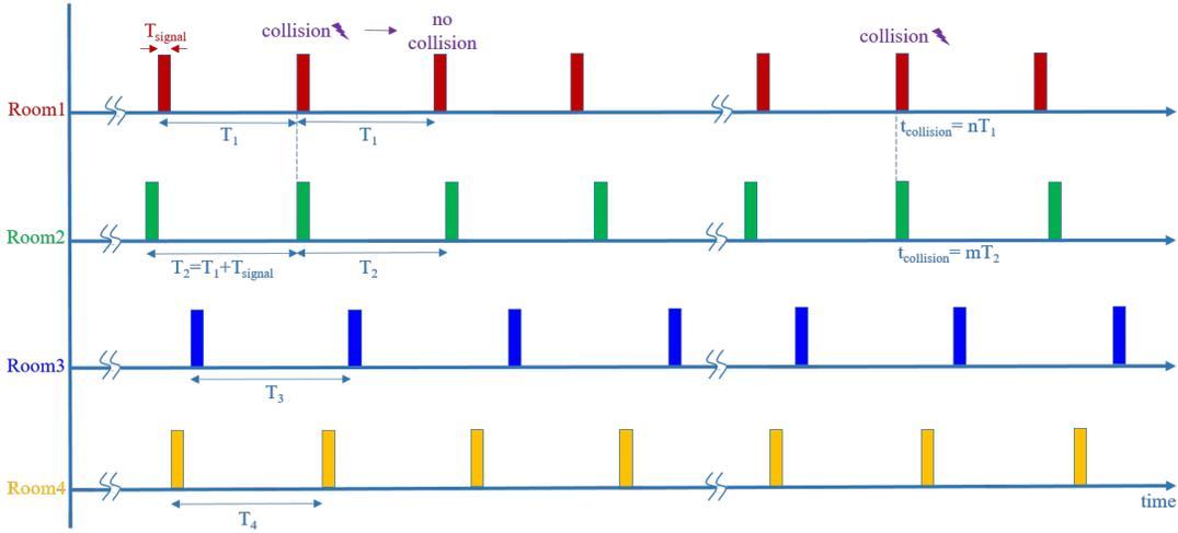
Fig. 10. Adjacent rooms have slightly different periods of emissions: no successive collisions occur, and the time between two collisions is maximized
