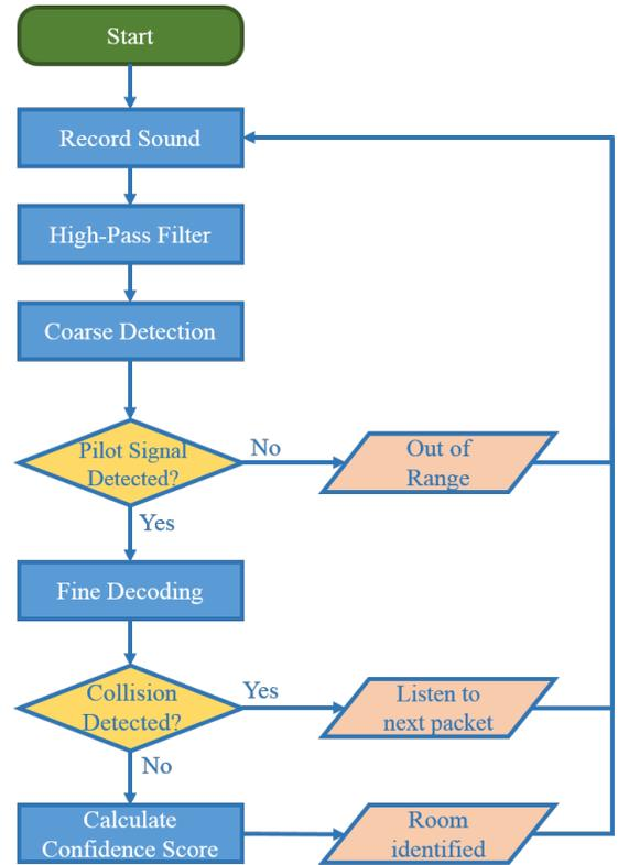
Fig. 8. Flow chart of the localization process
