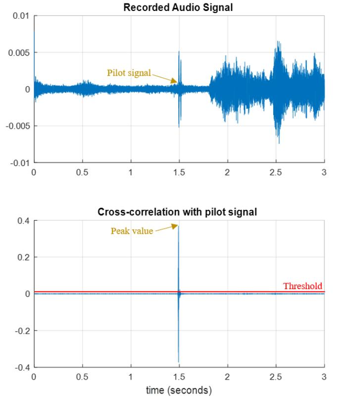
Fig. 6. The first plot shows the recorded audio signal. The second plot shows the result of its cross-correlation with the known pilot signal
