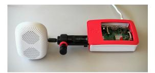
Figure 3. Prototype of the ultrasound motion sensor used for testing.
