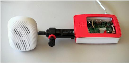
Figure 3. Prototype of the ultrasound motion sensor used for testing.
