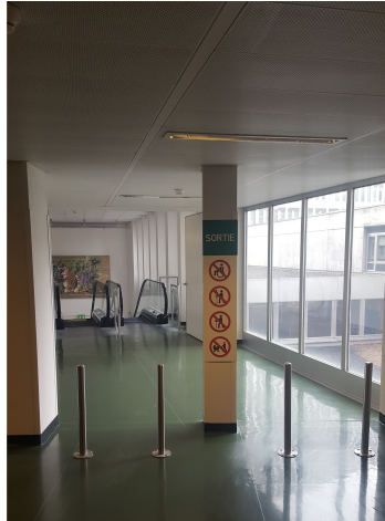
(c) Warning sign before an escalator leading to the exit, mentioning that it is not suitable for people using a cane or a wheelchair. No alternative route sign exists though.
