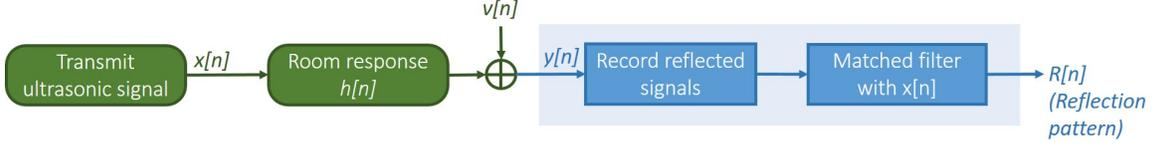
Figure 1. Obtaining the reflection pattern.
