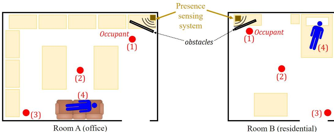
Figure 7. Tests' scenarios showing the occupant's position for the *occupied* frames: (1) close to the transmitter (standing/sitting), (2) at moderate distance (standing/sitting), (3) far from the system (standing/sitting), and (4) lying down. Obstacles are placed to simulate the NLOS case, and removed for LOS case
