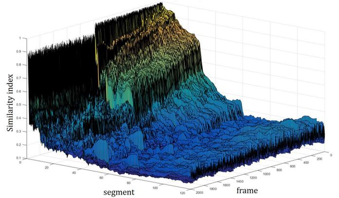
Figure 8. Similarity indices over segmented reflection patterns for vacant (frames 1-1000) and occupied environment (frames 1001-2000), case of high SNR, Room A, LOS.
