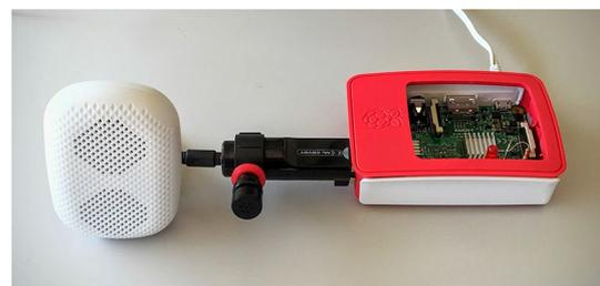
Fig. 7 Prototype of the ultrasound motion sensor used for testing
