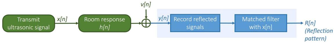
Fig. 4 Obtaining the reflection pattern
