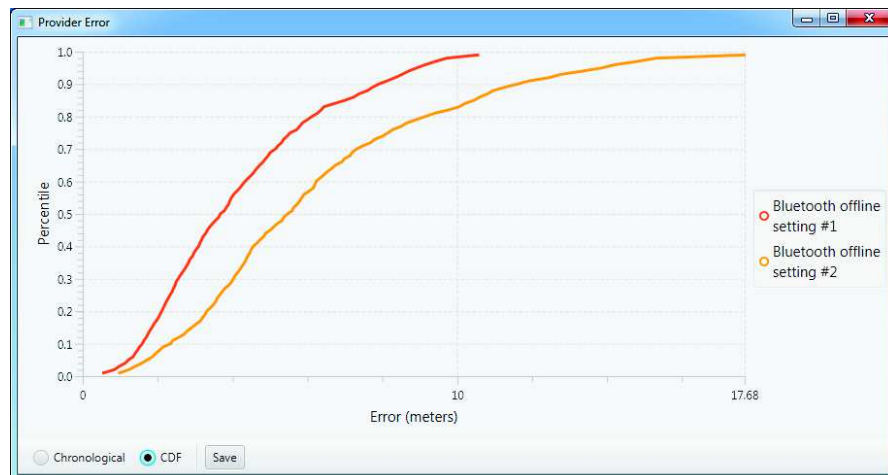
Figure 8.7. The CDF of the positioning error with two different parameter tunings, produced by GpmStudio.
