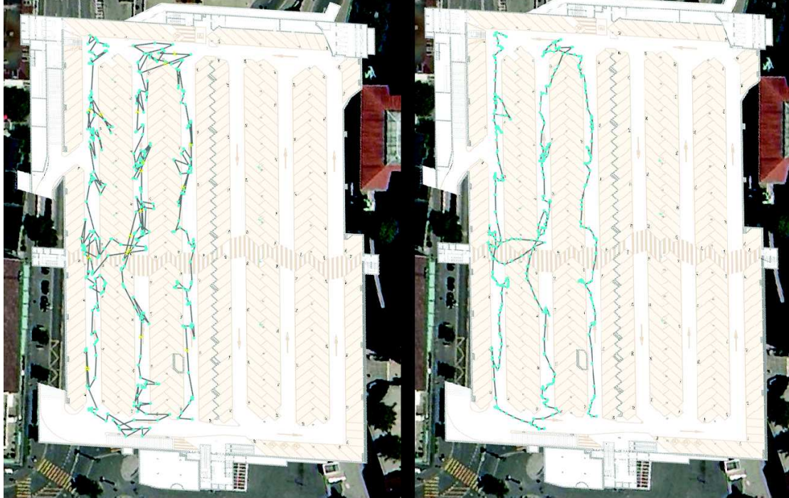
Figure 4.7. The estimated trajectory given by the unfiltered output (left image), and the filtered one (right image)
