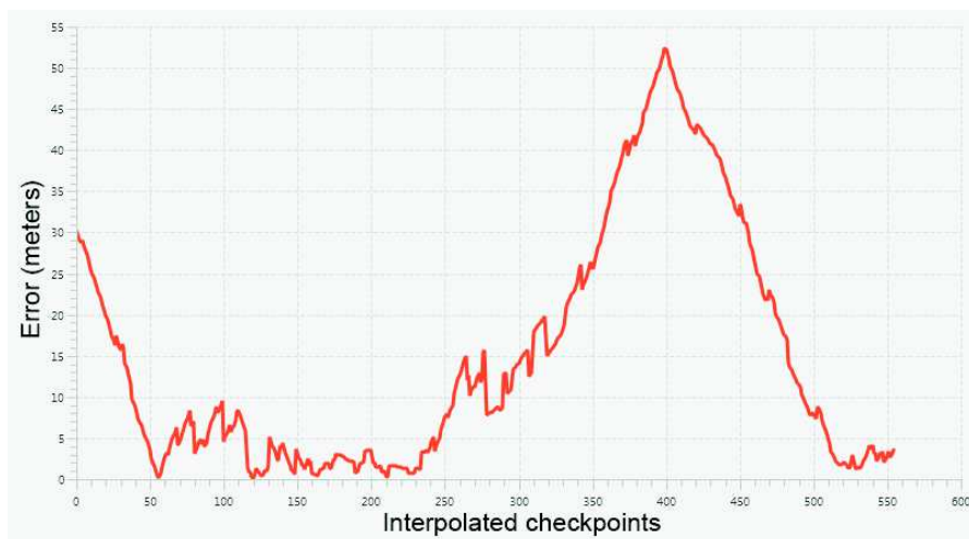
Figure 7.5. Error of a Bluetooth position provider along a path, as it changes over time
