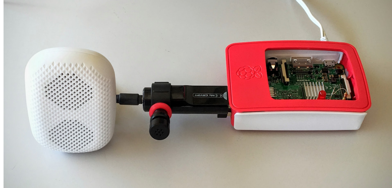
Figure 4.8: The implemented prototype comprises a commodity speaker and a microphone connected to a Raspberry Pi board.
