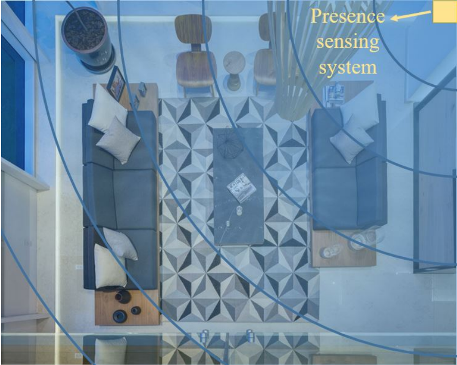
Figure 6.4: Segmenting the reflection pattern is equivalent to dividing the environment into segmented spaces (iteratively discarding the first i segments).
