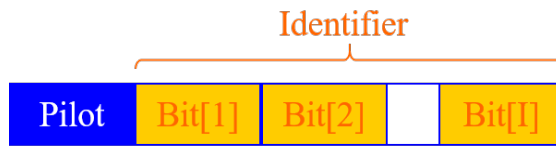
Figure 3.1: Design of the transmitted ultrasound packet
